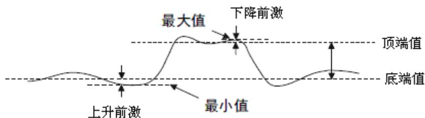
$$\text{下降前激} = \frac{\text{最大值} - \text{顶端值}}{\text{幅值}} \times 100\%$$
