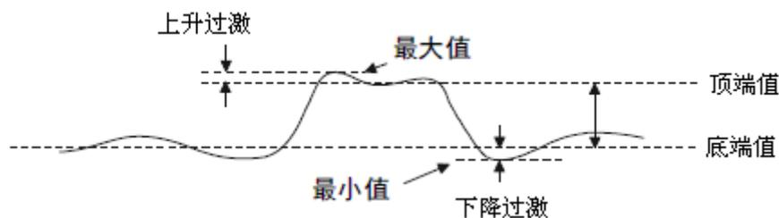
$$\text{上升过激} = \frac{\text{最大值} - \text{顶端值}}{\text{幅值}} \times 100\%$$
